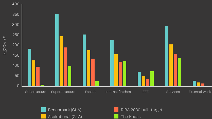
Graph 6: Life cycle embodied carbon (A1–A5 + B1–B5 + C1–C4) comparison with industry benchmarks
